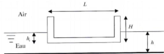
On prendra  $L = 10 \text{ m}$ ,  $l = 4 \text{ m}$ ,  $H = 5 \text{ m}$ ,  $m = 54000 \text{ kg}$ ,  $h = 4 \text{ m}$ ,  $\rho_{eau} = 1000 \text{ kg.m}^{-3}$ .
