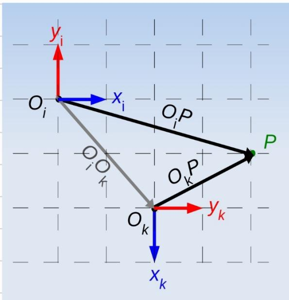
$$\begin{aligned} x_k &= -y_i \\ y_k &= z_i \\ z_k &= z_i \end{aligned} \quad \left. \begin{aligned} \vec{x}_k &= \vec{x}_i O - \vec{y}_i + \vec{z}_i O \\ \vec{y}_k &= \vec{x}_i + \vec{y}_i O + \vec{z}_i O \\ \vec{z}_k &= \vec{x}_i O + \vec{y}_i O + \vec{z}_i O \end{aligned} \right\} \text{Permet de trouver } {}^iR_k$$
